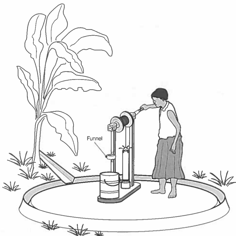
Figure 38 The Blair bucket pump. Source: Morgan (1990)
